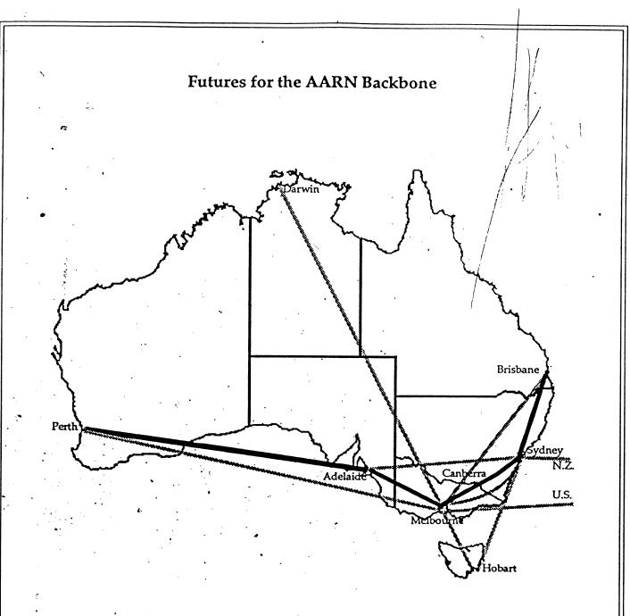
Increase bandwidth on trunk links - Megabit main trunk with additional 64K/144K ISDN links.
